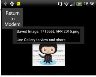
You can return to the Modem screen at any time during or after the reception of an MFSK image without affecting the image received. The "Saved image" message will advise the end of the image reception.
